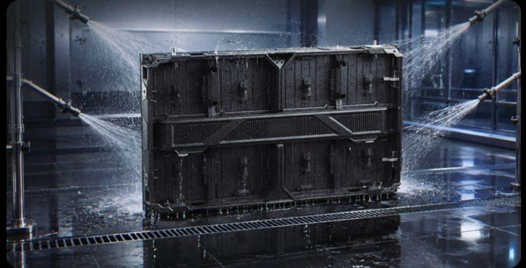
IP65 spray test from both sides: protected against water jets, not against high pressure.
