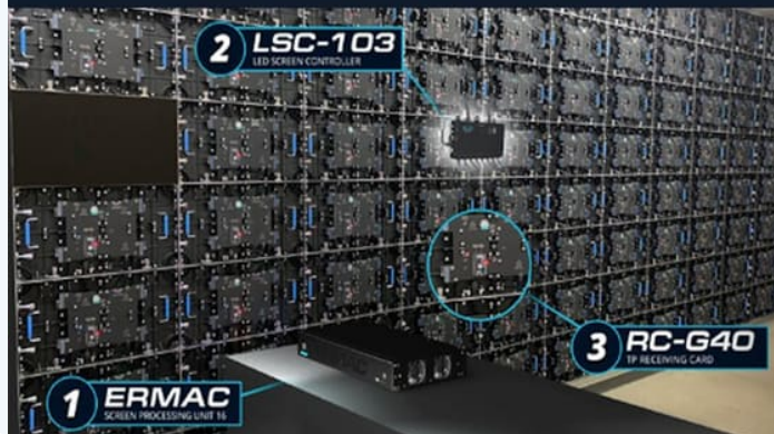
XF+ SERIES: PANEL, ERMAC SYSTEM COMPONENTS AND CABINET DIMENSIONS
